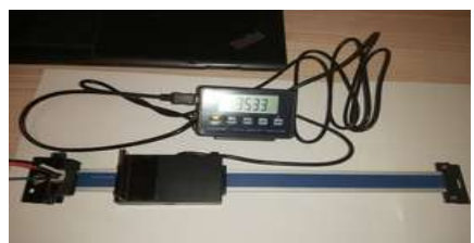
Testing setup with electronic ruler for optical sensors for displacement measurement.
