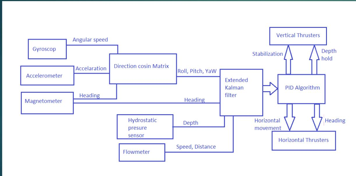
The signal bloc diagramme of AUV
