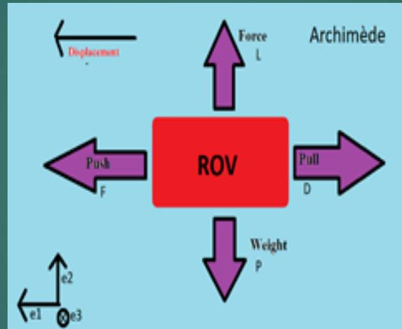
The underwater ROV body a) and the forces on the ROV body b)
