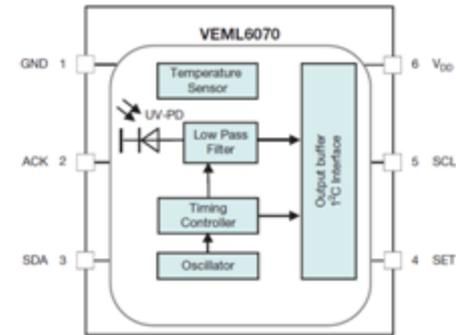
Figure 10. Block diagram of VEML6070 sensor.
