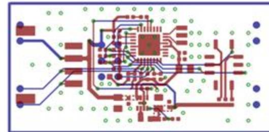
Figure 4. Prototype printed circuit board of Atmega 328 8-bit microcontroller adapter
