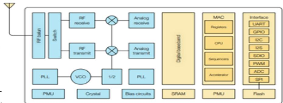
Figure 3. The functional block diagram of ESP8266 series
