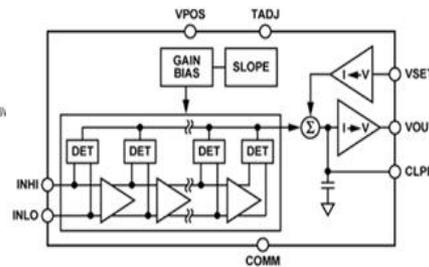
Figure 8. Block diagram of type AD8317
