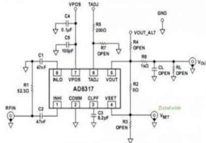
Figure 9. Prototype schematic AD8317
