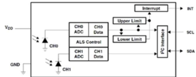
Figure 11. Block diagram of TSL2591 converter.
