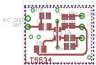
Figure 7. Prototype printed circuit board of LT5534
