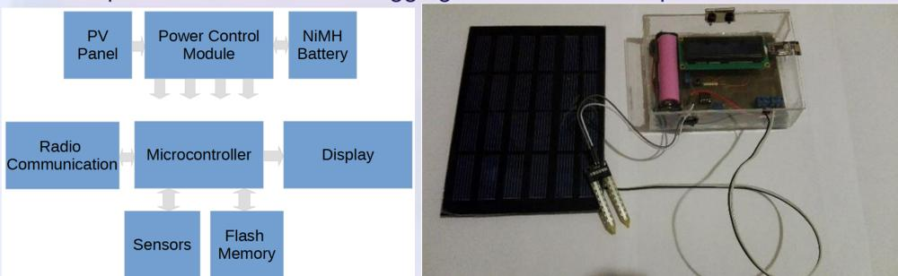
The proposed structure includes a 16 bit microcontroller, flash memory, communication module, LCD display, sensors and analog electronics that implements power control for charging the NiMH battery from solar panel and supplying the entire system.
