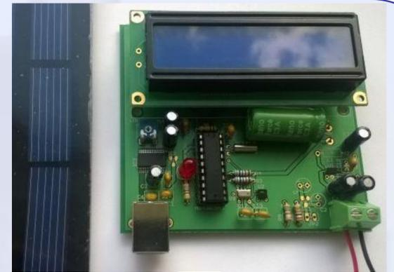
Structure of a microcontroller-based datalogger module with solar panel supply and energy storage (a) and its implementation with 10Farad supercapacitor as energy storage (b).
