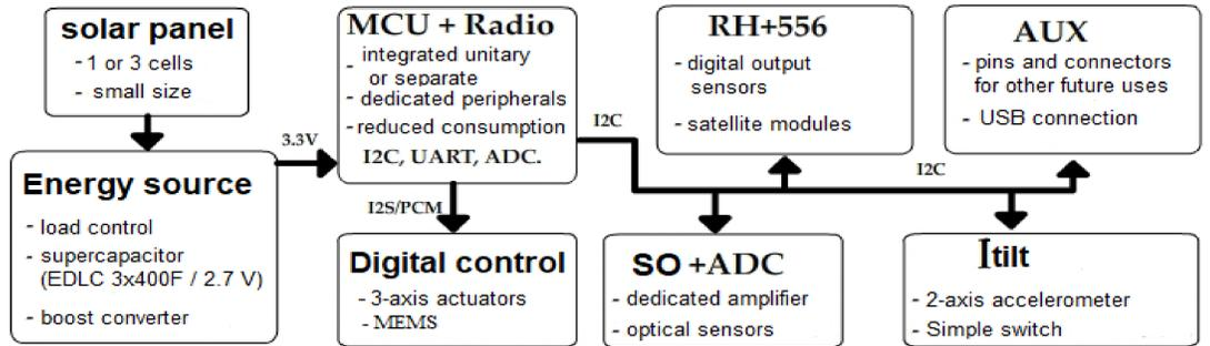
Figure 1. Simplified block diagram of the system.
