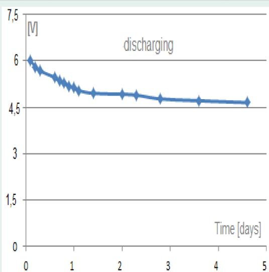
Figure 10. Discharge the 3 EDLC battery
