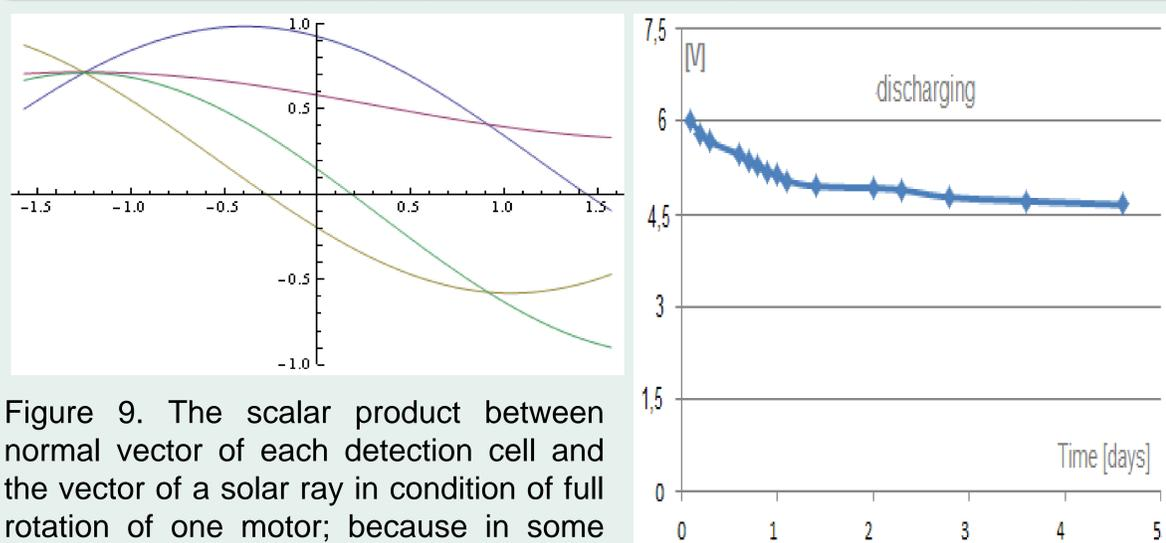
Figure 9. The scalar product between normal vector of each detection cell and the vector of a solar ray in condition of full rotation of one motor; because in some point the 4 curves are intersecting that point represent the optimal position.
