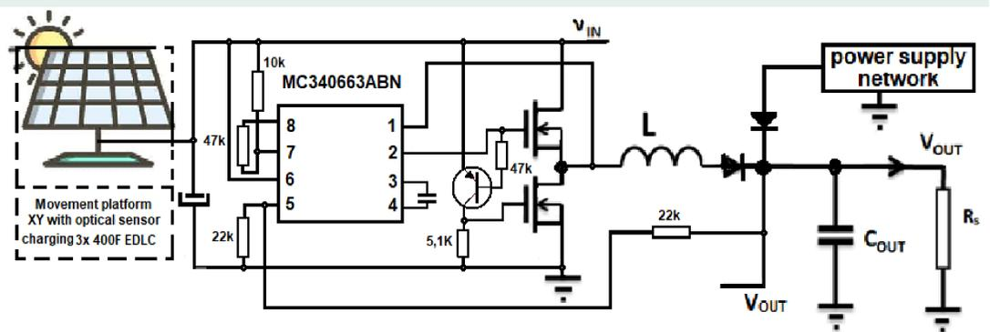
Figure 7. Experimental circuit with high reliability hybrid power supply
