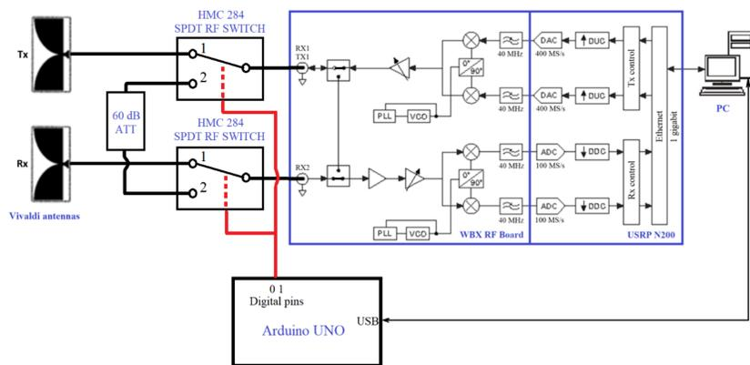
Fig. 1. Experimental setup – block diagram.
