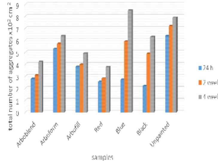
By the end of the experiment, the bacterial monolayer (known as biofilm) was maintained for 2 weeks for liquid wood samples, except for Arboblend which remained in the monolayer for 3 weeks). The samples covered with antifouling paint had a different evolution due to the appearance of rust spots on the surface of the samples in compartment C2 where the presence of oxygen accelerated the oxidation reaction of the naval steel.
