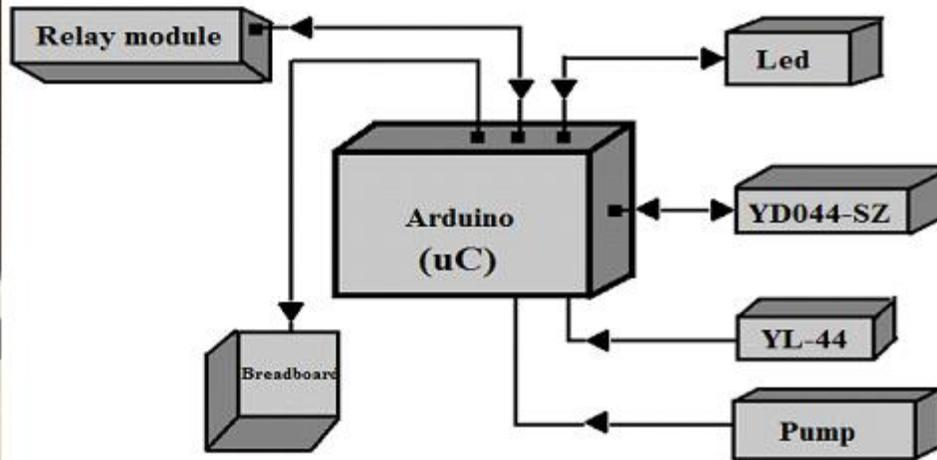
The microcosms system for monitoring, block diagram of water monitoring system
