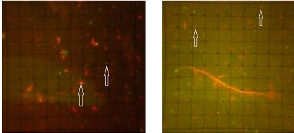
Visualization of living (green) and dead (red) organic fractions from naval steel sample and liquid wood sample
