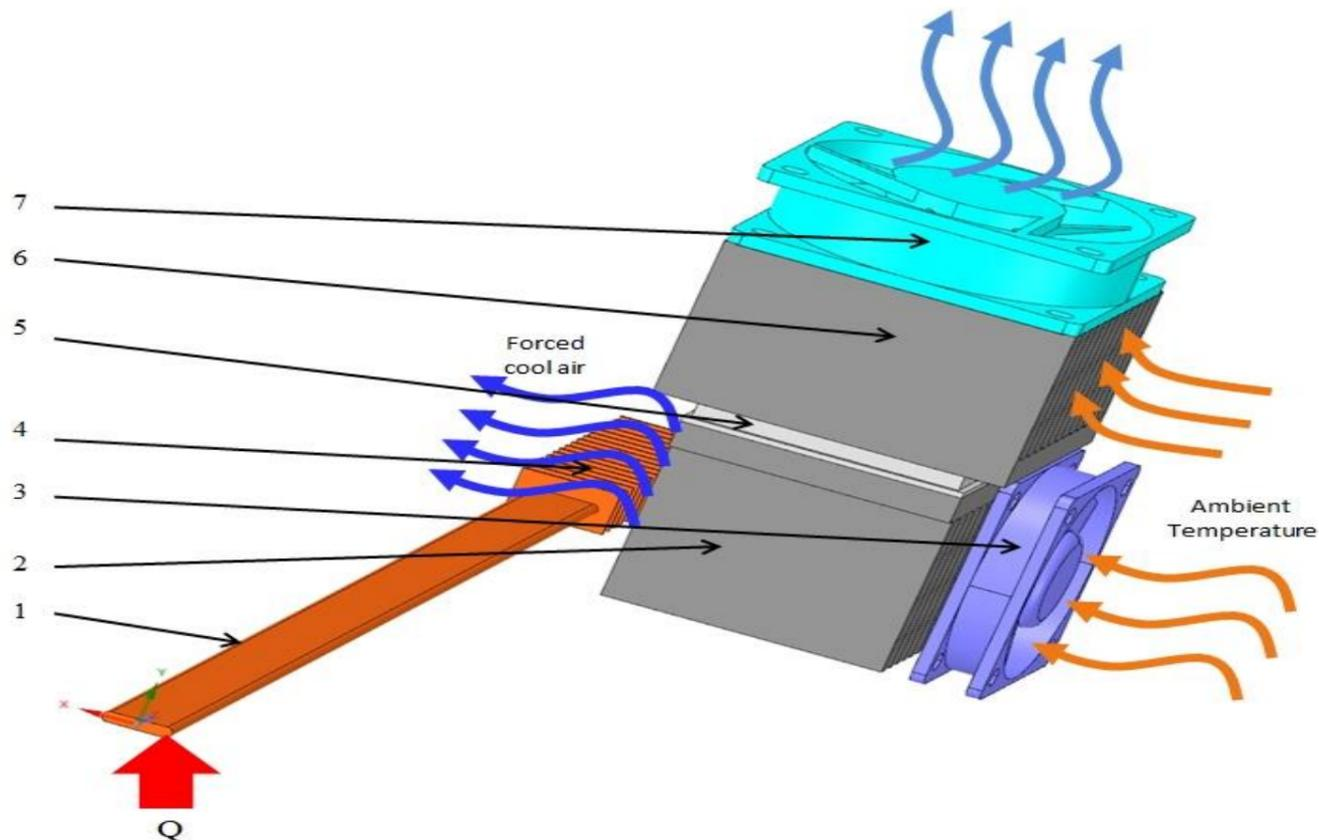
Figure 3. Cooling of the condensation zone by inverted Seebeck effect
