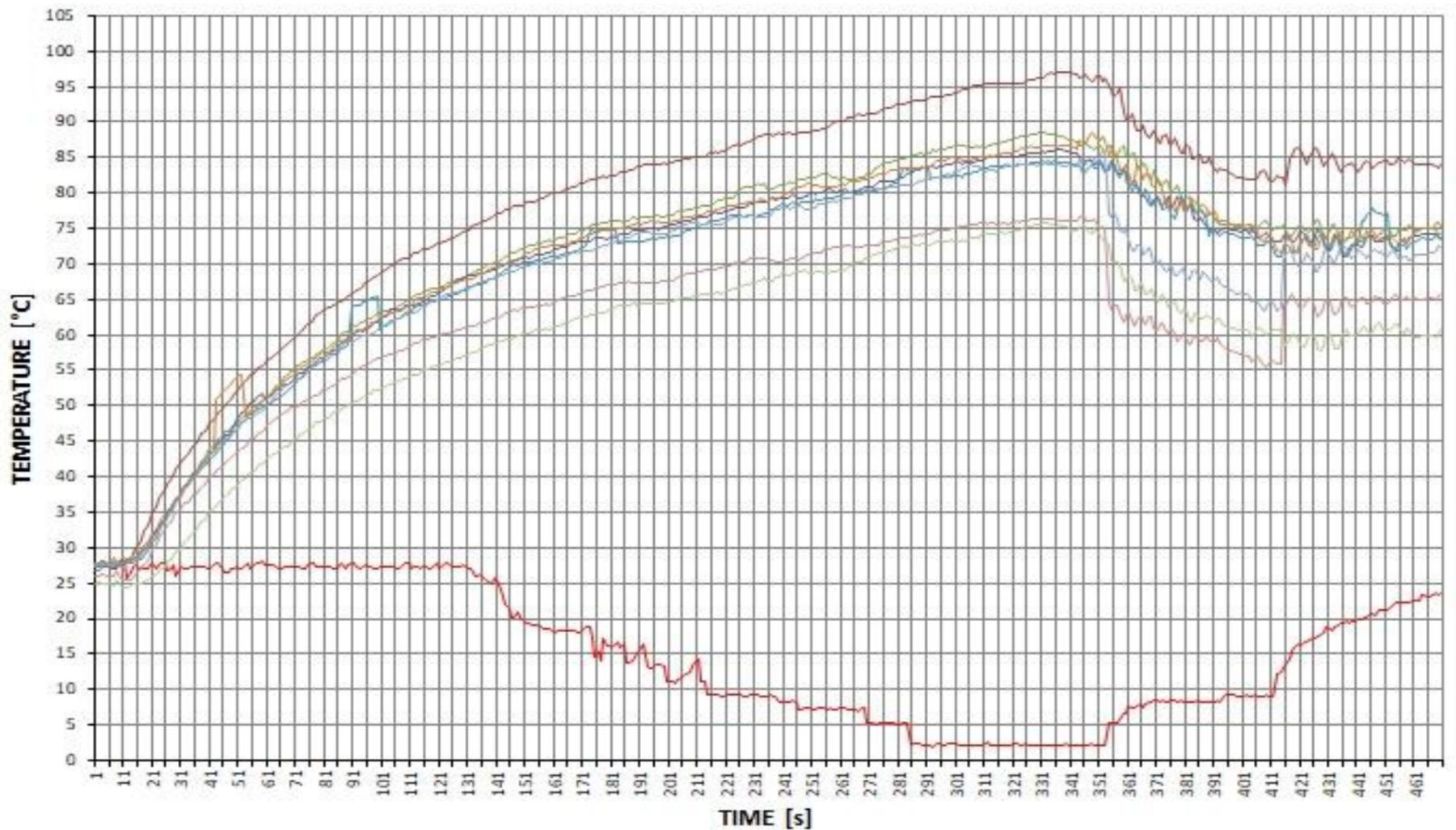
Figure 4. The temperature variation on the three areas of the FMHP and on the radiator cooled through the inverted seebeck effect.
