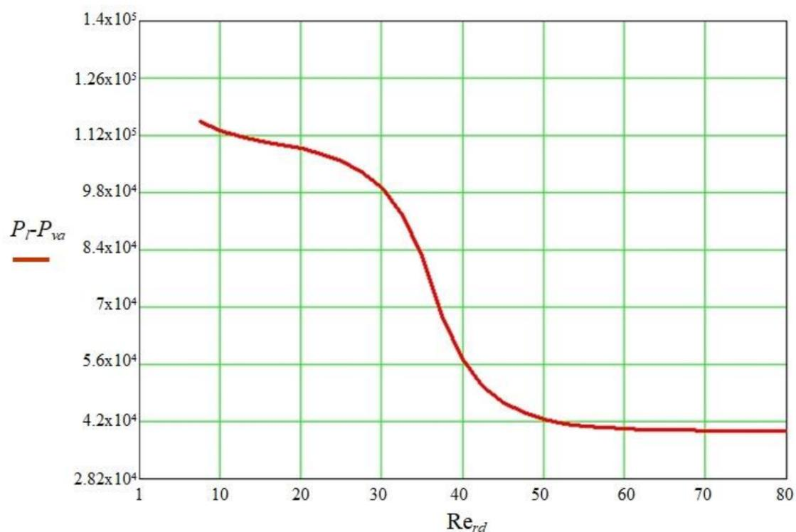
Figure 2. The variation graph of  $P_l - P_{va}$  depending on  $Re_{rd}$  la  $T_l = 85^\circ\text{C}$
