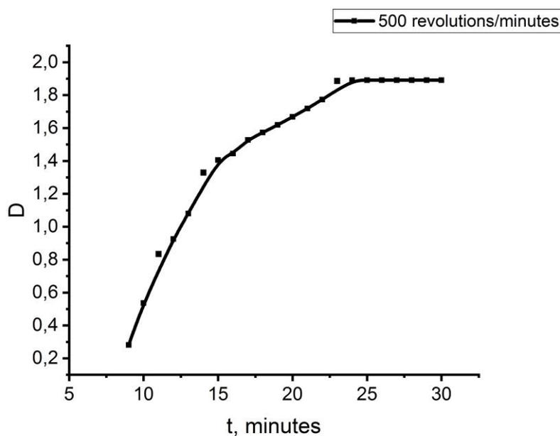
Fig. 2. Dependence of the optical density of the samples on the centrifugation time for centrifugation frequency of 500 rpm<sup>6</sup>
