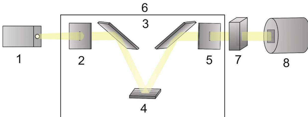
Fig. 1. Setup for measuring the optical density of the samples: 1 - filament lamp of iodine cycle with a stabilizer, 2 - the entrance slit, 3 - the system of rotating mirrors, 4 - the diffraction mirror, 5 - the output slit, 6 - monochromator MUM-01, 7 - cuvette with the sample, 8 - radiation receiver<sup>22</sup>
