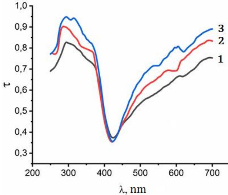
Fig. 5. The dependence of the transmittance of the samples on the wavelength for particles of different size: 1) 920 nm, 2) 456 nm, 3) 89 nm
