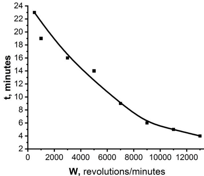
Fig. 3. Dependence of the deposition time of the particles on the rotation speed of the centrifuge<sup>22</sup>
