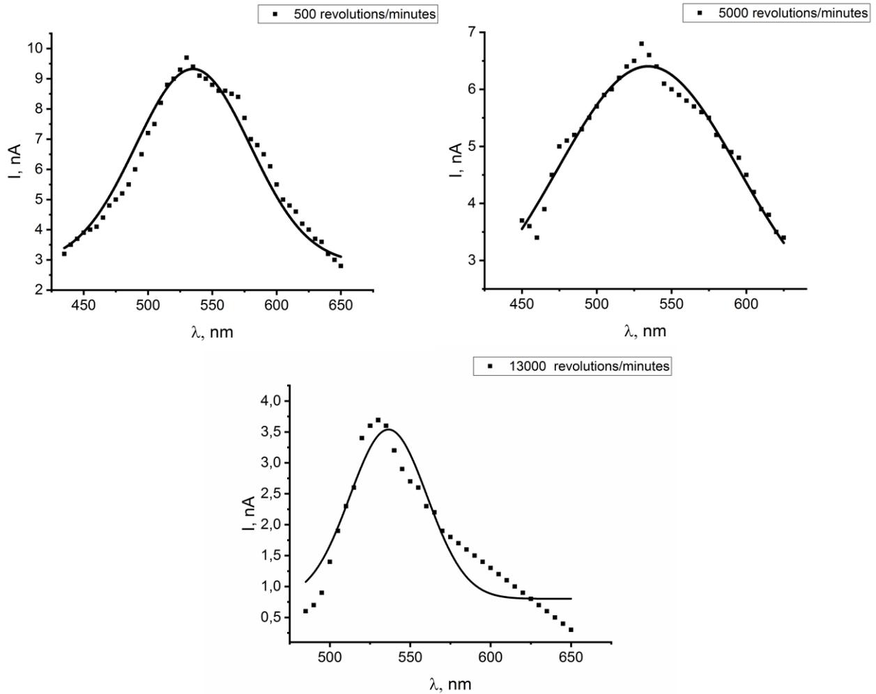
Fig. 6. Spectrum of luminescence for different rotation speed of the centrifuge<sup>22</sup>
