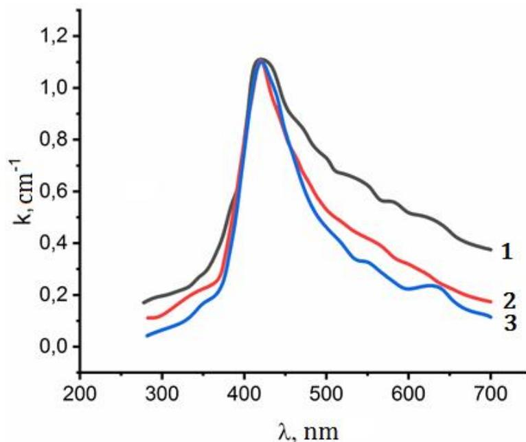
Fig. 4. Dependence of the absorption index of the samples on the wavelength for the centrifugation frequency: 1) 500 rpm, 2) 5000 rpm, 3) 13000 rpm
