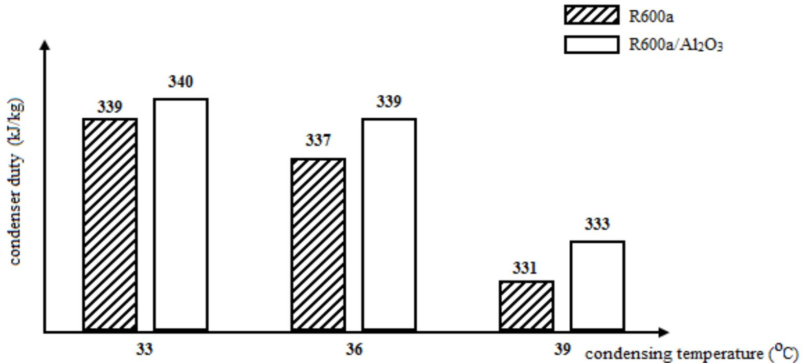
Figure 4 Working input versus condensing temperature
