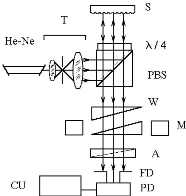
Fig. 2. Experimental arrangement for measuring the degree of arbitrary surface roughness:
