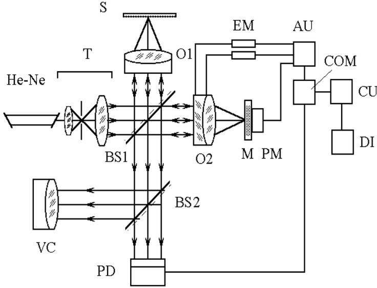
Fig. 1. Experimental arrangement for measuring the degree of low-reflectance surface roughness:
