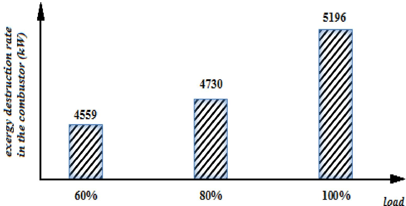
Figure 5 – Influence of load variation on the combustor efficiency
