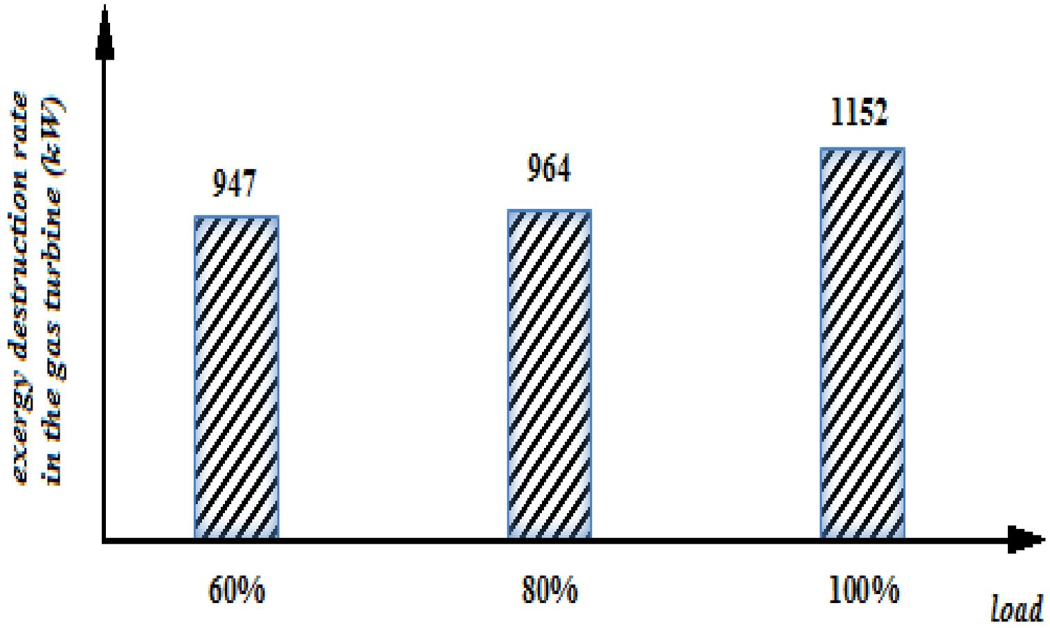
Figure 8 – Influence of load variation on the exergy destruction rate in exhaust gases
