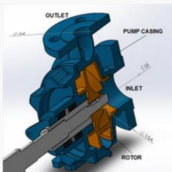
Figure 1. The CAD geometry of the pump on subject
