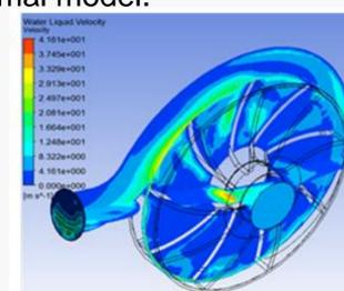
Figure 5. Water velocity calculated fields for the optimal model
