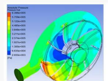
Figures 6. Absolute pressure fields for the optimal model
