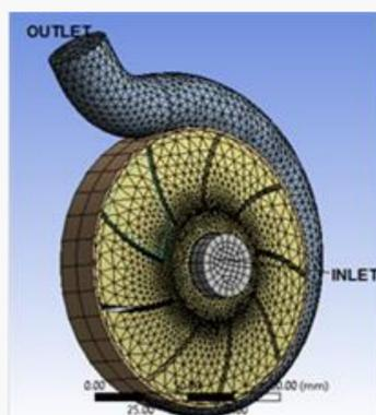
Figure 2. The finite volumes mesh
