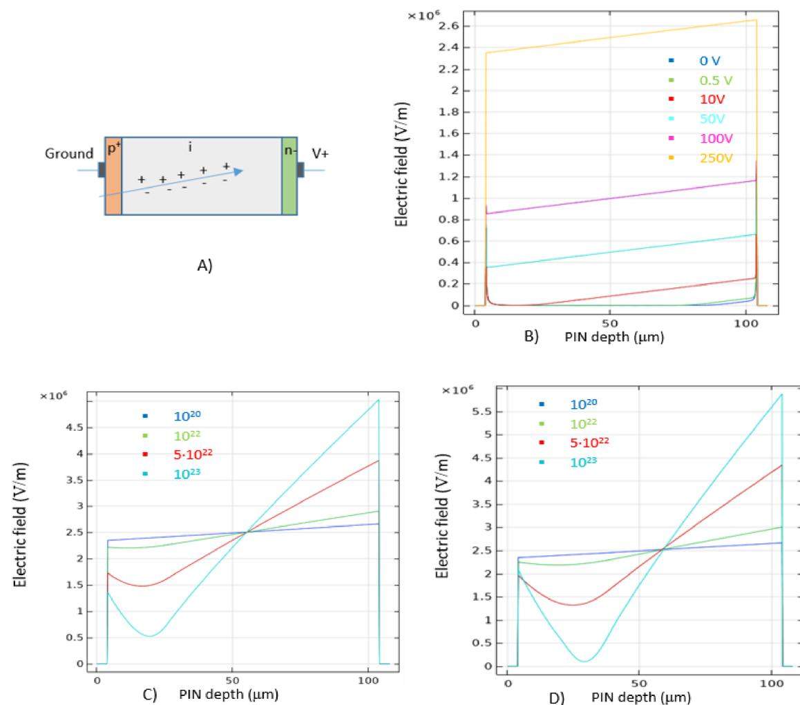
A) The structure of the PIN diode. B) Electric field distribution inside the PIN diode for several reverse bias voltage applied, no radiation. C)-D) Electric field distribution inside the PIN diode for different extrinsic generation rates (expressed in  $1/\text{cm}^3\text{s}$ ) when the length that produced electron-hole pairs by radiation is 26  $\mu\text{m}$  (C) and 38  $\mu\text{m}$  (D) (simulation with Comsol Multiphysics).
